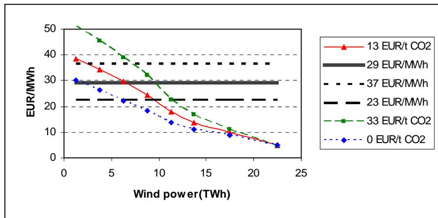
Figure 4. Sensitivity analysis. Variations of CO2 and wind power production costs.
