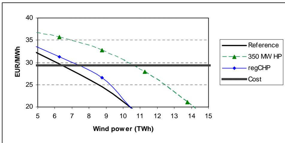
Figure 3. Marginal benefit of wind power in flexible versus non-flexible energy systems.
