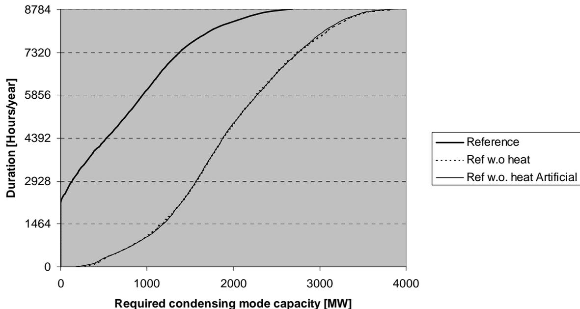
Figure 8: Duration curve for the reference system and for system without heat demand and thus heat-tied CHP generation with 2004 annual wind variation curve and artificial annual variation curve for wind power.
