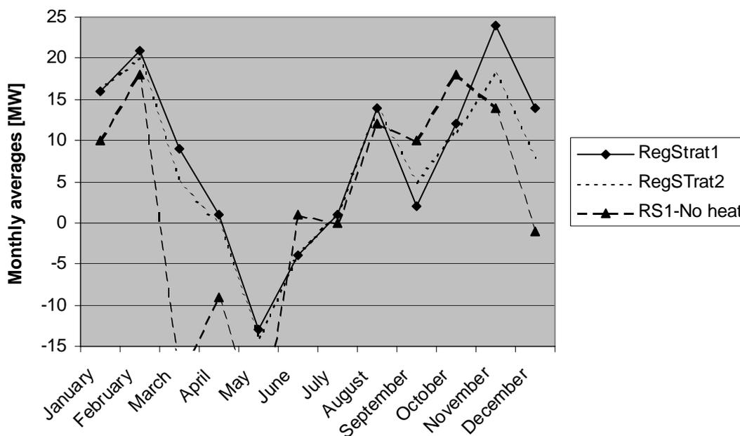
Figure 6: Change in average monthly condensation-based power generation with the artificial yearly wind distribution curve with Regulation Strategies 1 and 2 and in a situation without any heat demand covered by CHP. Positive values indicate reduced condensation-
