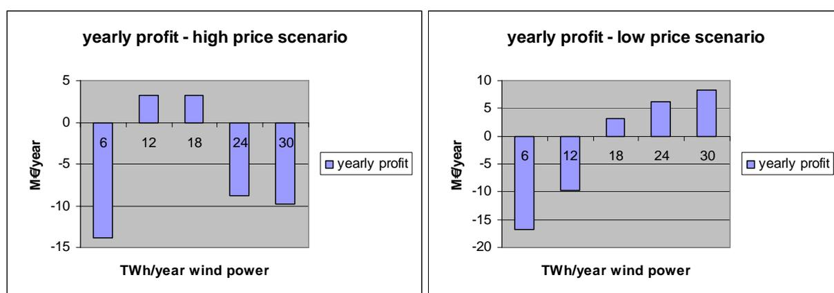
Figure 5. Profit of increasing interconnector capacity with 1000 MW.
